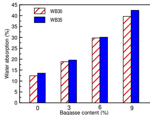
Fig. 4. Effect of sugarcane bagasse content on water absorption of brick samples.
