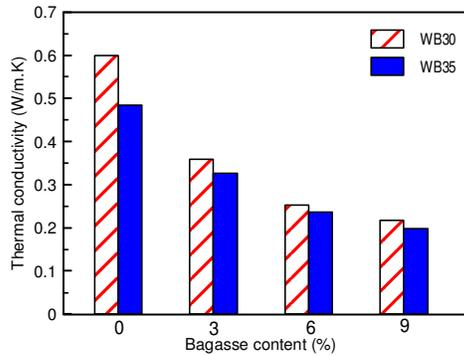
**Fig. 5.** Effect of sugarcane bagasse content on thermal conductivity of brick samples.
